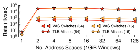
Figure 9: Rate of VAS switching and TLB misses for GUPS executed with SpaceJMP, averaged across 16 iterations. TLB tagging is disabled. A larger window size would produce a greater TLB miss rate using one window.
